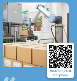
At L'Oréal India's Pune plant, for example, manual end-of-the-line operations involved operators lifting approximately 8,500 kg of product per 8-hour shift. Concerned about the ergonomic risk, L'Oréal India deployed two UR10s on palletizing tasks, enabling the cosmetics giant to improve worker health and safety and improving overall equipment effectiveness in the plant by 5%, thanks to the time saved in pallet replacement.
