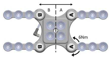
When the four arms are adjusted to preferred angles, it is recommended to add the accompanied arrow stickers. This allows for easy realignment and exchanging between different work items.
